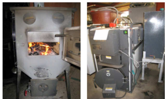
Fig. 1. The tested commercial scale stove and boiler.
