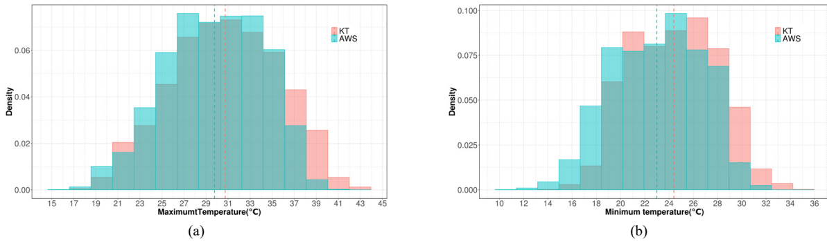
Fig. 12. Differences in the distribution of (a) daily maximum temperature and (b) daily minimum temperature between Korea Meteorological Administration's AWS and KT observational data
