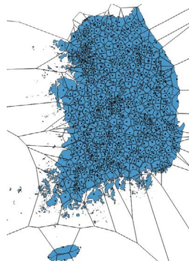
Fig. 3. Thiessen network of meteorological station
